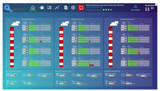
The emission computer determines the operating status of the object using analog, binary and digital signals supplied to it, and then can transmit data via Ethernet to another unit.
